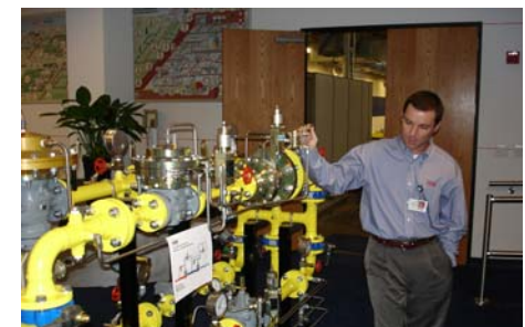
Natural Gas skid—city gate, district station, commercial/industrial and distribution regulators—used to stage live operation, maintenance, and troubleshooting demonstrations.
