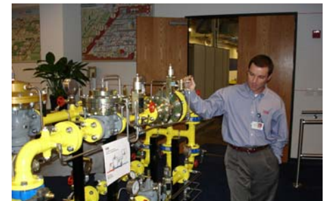
Natural Gas skid—city gate, district station, commercial/industrial and distribution regulators—used to stage live operation, maintenance, and troubleshooting demonstrations.
